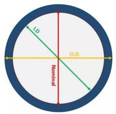
1" Lockrod means 1" pipe size 1.32" O.D. Tubing
